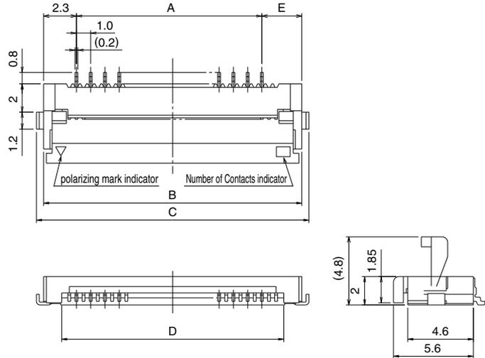
Note 1 : The coplanarity of each terminal lead within specified dimension is 0.1mm Max.
