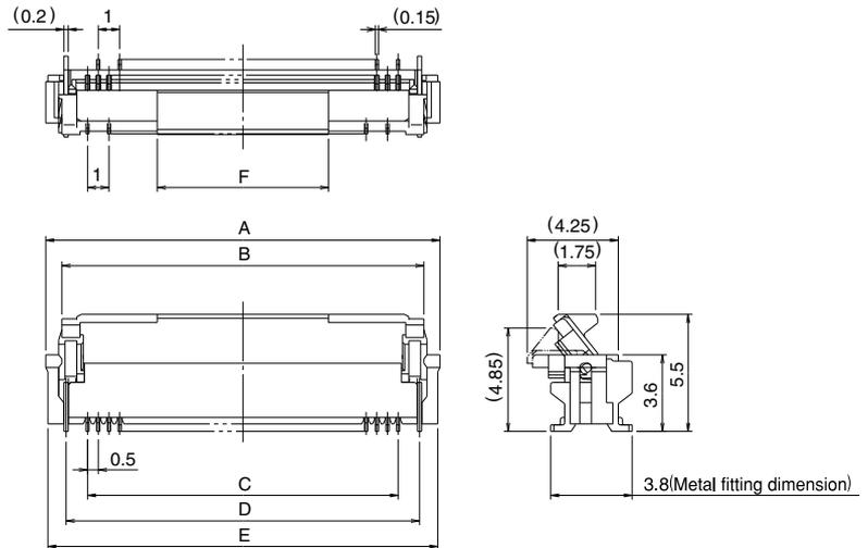
Note 1 : The coplanarity of each terminal lead within specified dimension is 0.1mm Max.
