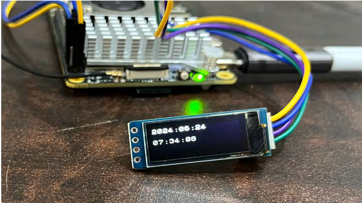
Fig. 5.24: Date & Time on 128x32 OLED
