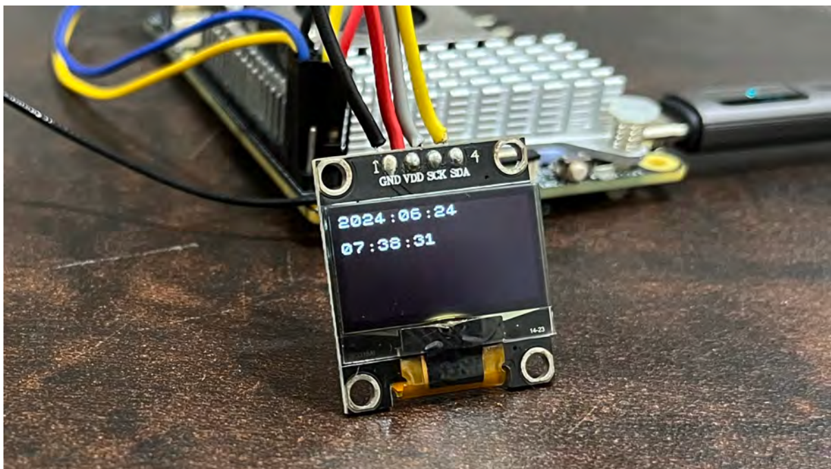
Fig. 5.23: Date & Time on 128x64 OLED
