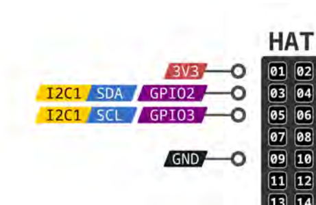
Fig. 5.15: BeagleY-AI I2C pinout
