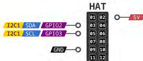
Fig. 5.25: BeagleY-AI I2C pinout (5V)
