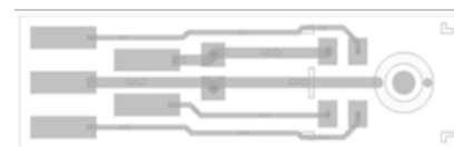
Figure 2. EV_ICS-40618-FX Board Layout (Top View) 12 mm x 3.6 mm
